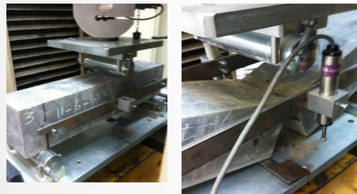
Figure 1. Test set-up of the three-point bending test
