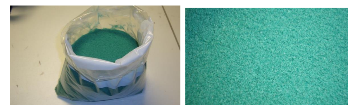
Figure 8. linear low density polyethylene (LLDPE) powder add to high performance concrete with different percentages
