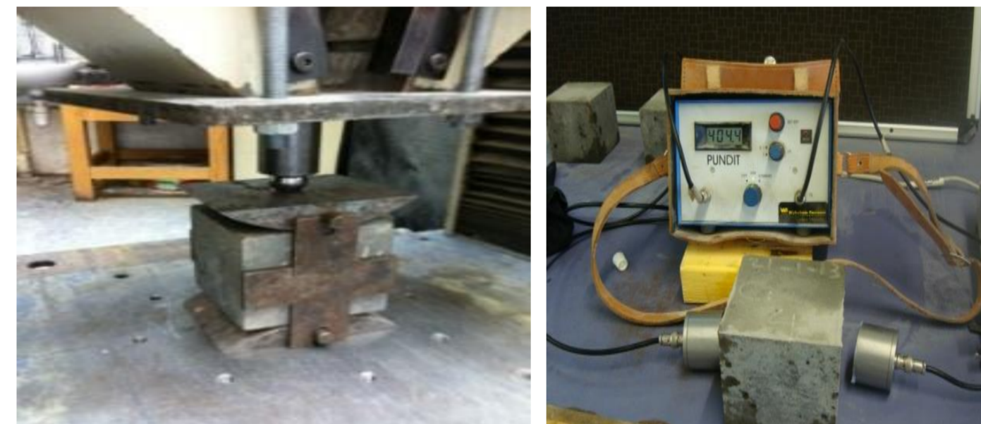
Figure 6. : Splitting tension test Figure 7. Ultrasonic testing
